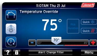
The exclusive "Quick Heat and Cool" feature allows you to "speed up" either the heating or cooling mode by temporarily putting your system at the highest capacity.
