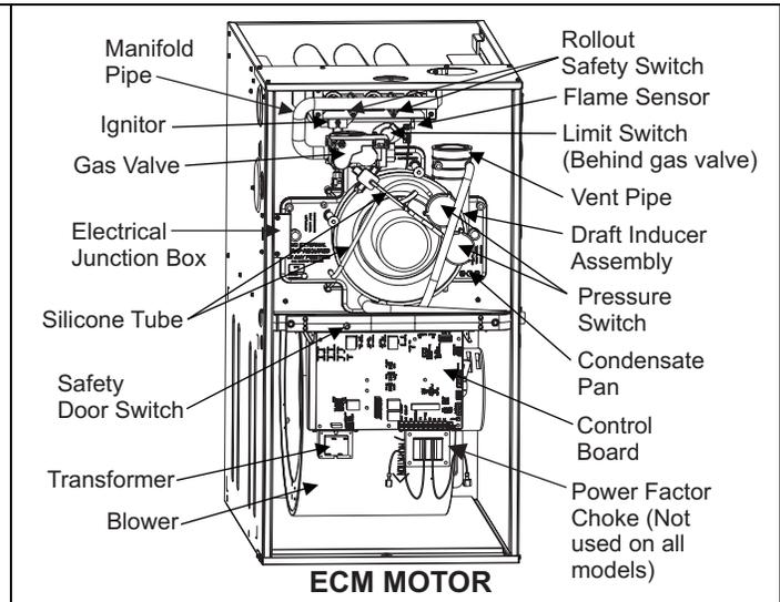
FIGURE 6: Component Location - 97% Modulating ECM Models
