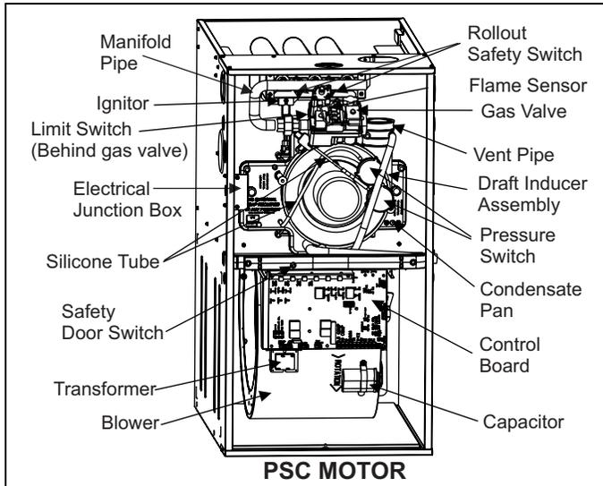
FIGURE 5: Component Location - 97% Modulating PSC Models
