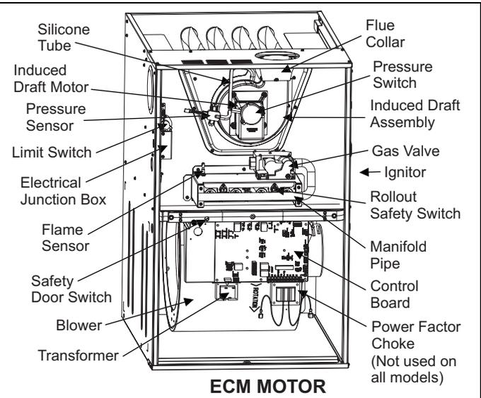
FIGURE 4: Component Location - 80% Modulating ECM Models
