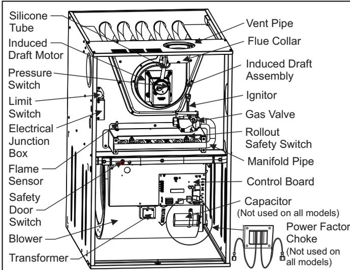
FIGURE 1: Component Location - 80% Single & Two Stage Models
