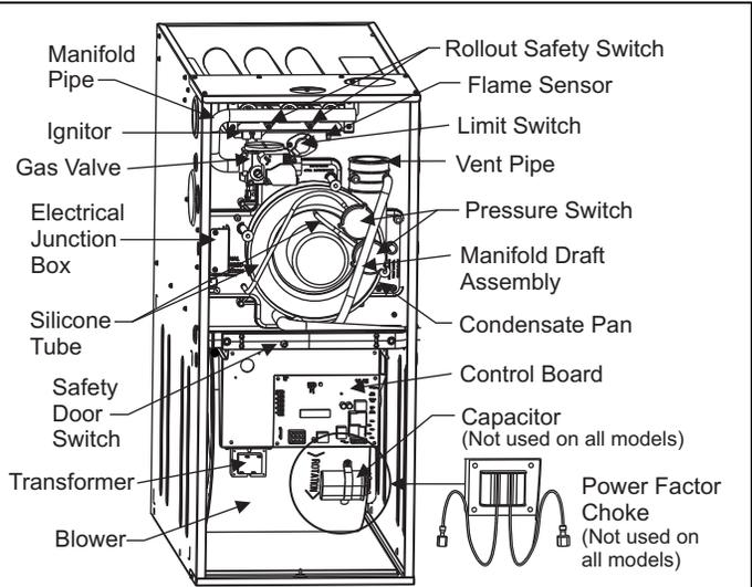
FIGURE 2: Component Location - 95% Single & 96% Two Stage Models
