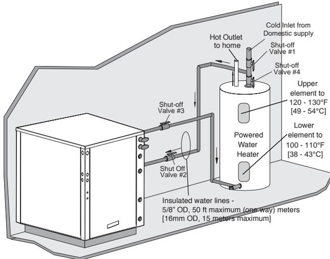
Typically a single tank of at least 52 gallons (235 liters) is used to limit installation costs and space. However, a dual tank, as shown in Figure 4, is the most efficient system, providing the maximum storage and temperate source water to the HWG.
