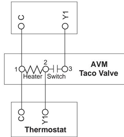
Figure 7: Taco SBV Valve Wiring
