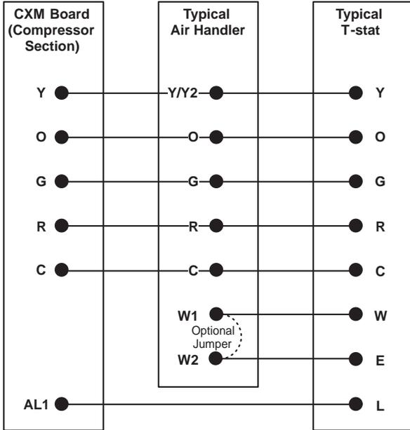
Figure 28c: Typical Thermostat Wiring, Two-Stage Units (3 Heat/2 Cool)
