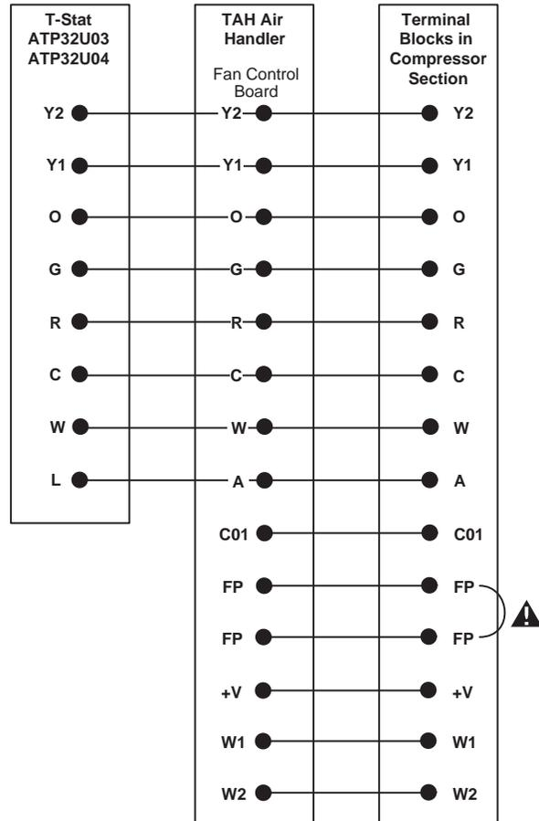
**⚠ IMPORTANT:** Violet jumper from FP to FP on Terminal block 2 in compressor section must be removed when unit is installed with TAH air handler or when FP2 sensor is field installed on existing air handler.
