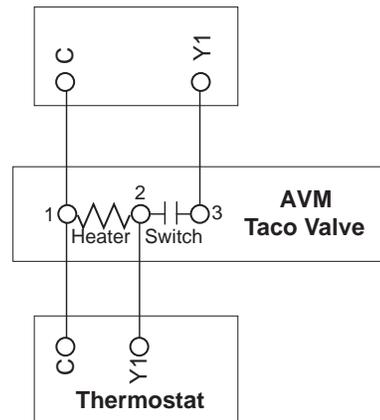
Figure 26: Taco SBV Valve Wiring
