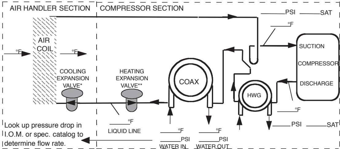
\*Cooling expansion valve meters in the cooling mode, and bypasses in the heating mode.
