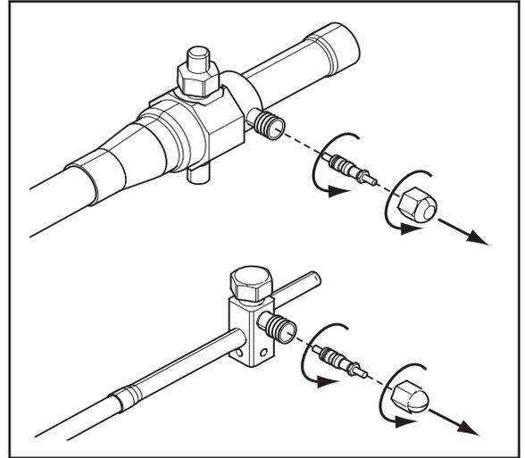
**STEP 3** - Purge the refrigerant lines and indoor coil with dry nitrogen.
