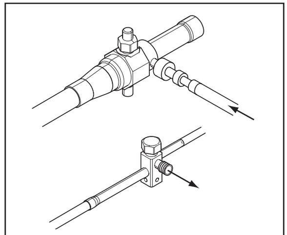
**STEP 4** - Wrap a wet rag around the valve body to avoid heat damage and continue the dry nitrogen purge.
