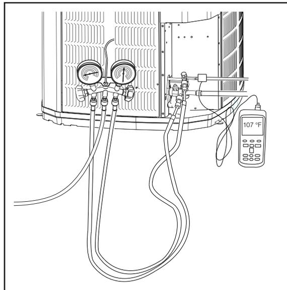
**STEP 5** - Use the final subcooling value, refrigerant temperature and pressure from STEP 4, to determine the proper liquid gage pressure using Table 14.2.
