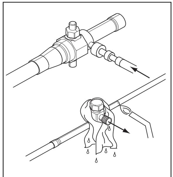
**STEP 5** - Replace the pressure tap valve cores after the service valves have cooled.
