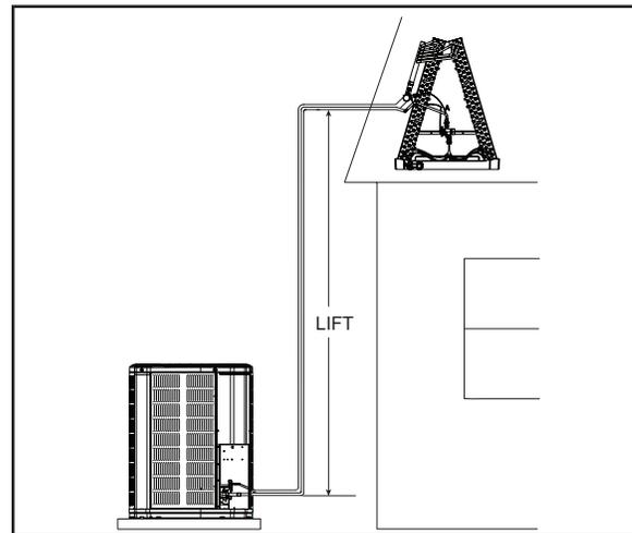
**STEP 2** - Determine the final subcooling value using total Line Length and Lift measured in STEP 1 and the charts below.
