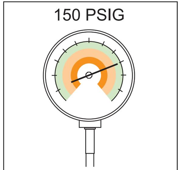
**STEP 2** - Check for leaks by using a soapy solution or bubbles at each brazed location.
