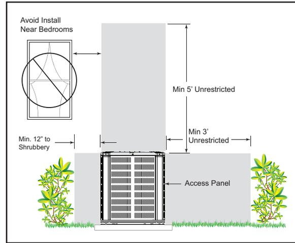
Position the outdoor unit a minimum of 12" from any wall or surrounding shrubbery to ensure adequate airflow.
