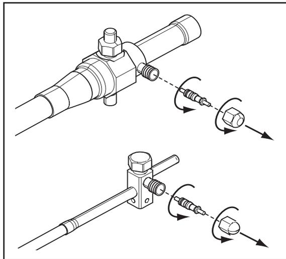
**STEP 3** - Purge the refrigerant lines and indoor coil with dry nitrogen.
