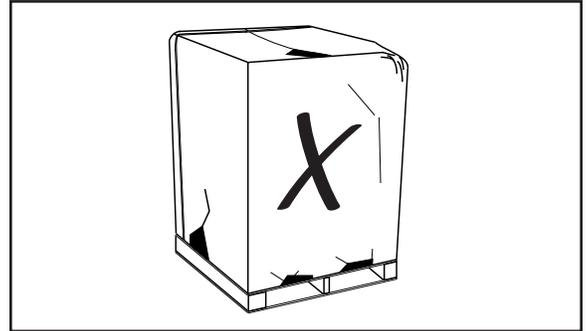
**STEP 2** - To remove the unit from the pallet, remove tabs by cutting with a sharp tool.
