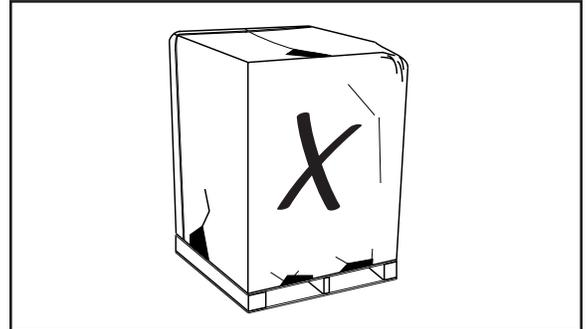
**STEP 2** - To remove the unit from the pallet, remove tabs by cutting with a sharp tool.
