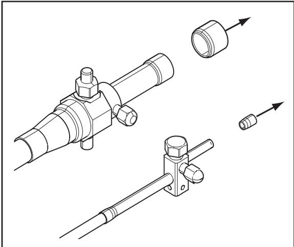
**STEP 2** - Remove the pressure tap cap and valve cores from both service valves.
