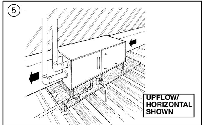
The furnace may be placed horizontally in a crawl space on a pad or other noncombustible material which will raise the unit for sufficient protection from moisture. **The furnace must be supported at both ends and the middle when installed horizontally.**
