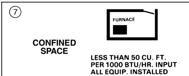
1. All air from inside the building as in Figure 8: The confined space shall be provided with two permanent openings communicating directly with an additional room(s) of sufficient volume so that the combined volume of all spaces meets the criteria for an unconfined space. The total input of all gas utilization equipment installed in the combined space shall be considered in making this determination. Refer to Table 2 for minimum open areas requirements.
