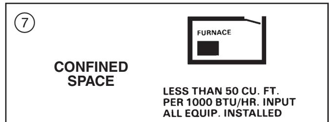
1. All air from inside the building as in Figure 8: The confined space shall be provided with two permanent openings communicating directly with an additional room(s) of sufficient volume so that the combined volume of all spaces meets the criteria for an unconfined space. The total input of all gas utilization equipment installed in the combined space shall be considered in making this determination. Refer to Table 2 for minimum open areas requirements.
