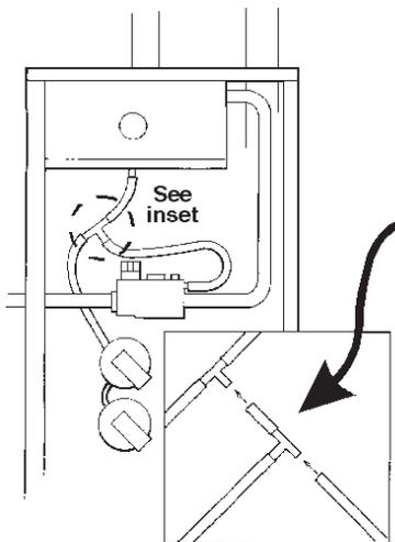
Separate the tube at the unit Tee and reconnect with a short piece of field supplied tube and another Tee with the "U" Manometer attached. Be sure to reconnect unit tubing to original position after testing the manifold pressure!
