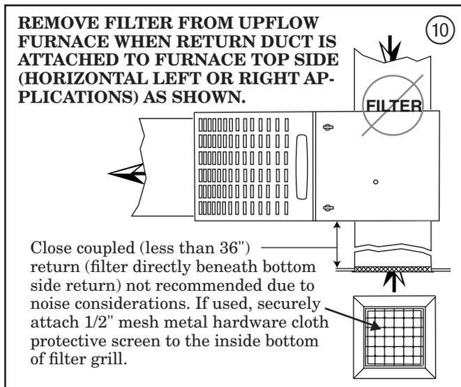
Close coupled (less than 36") return (filter directly beneath bottom side return) is not recommended due to noise considerations.
