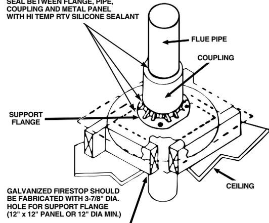
GALVANIZED FIRESTOP SHOULD BE FABRICATED WITH 3-7/8\"/>
