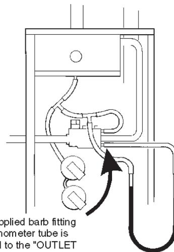
Field supplied barb fitting with manometer tube is attached to the "OUTLET PRESSURE TAP" on the outlet side of the gas valve.
