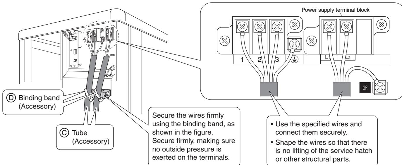
Observe the notes mentioned following when wiring to the power supply terminal block.
